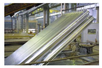
Hot-dip galvanizing, also known as dip galvanizing, is a widely used method of protecting steel structures from corrosion.
